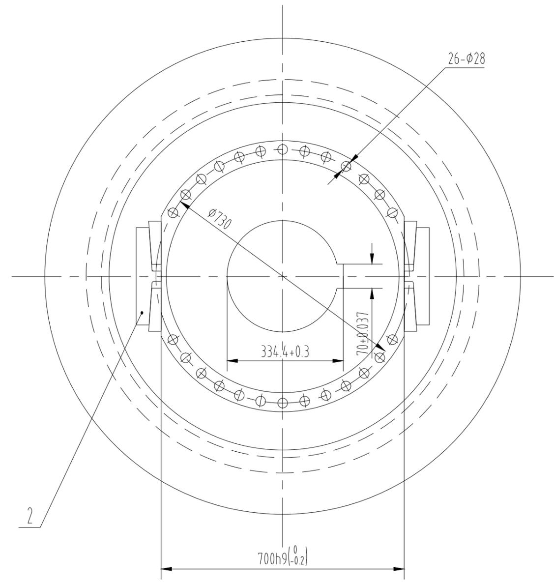
BOLT TIGHTENING TORQUE IN 660 Nm
