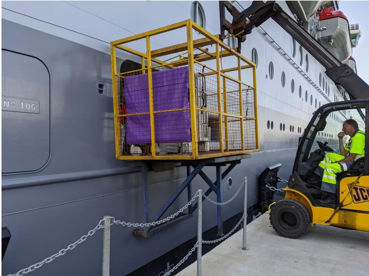
Once the carts were loaded, the basket was lowered to the ground 5 meters from the ship. The carts were then removed and staged in groups of 2. Forklifts then transported them to the terminal.
