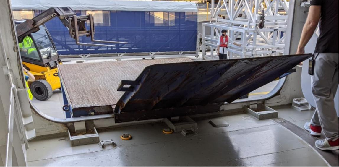
In Portsmouth, this basket was used to take carts off the ship using this boom equipped forklift. This basket could be used below pier level as tides required. Three carts fit easily.
